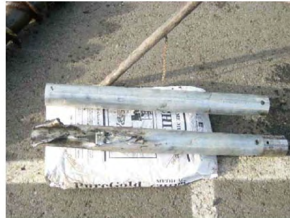
Photo 2. New Osterberg soil coring device (top) and sampler damaged by subsurface rocks.
