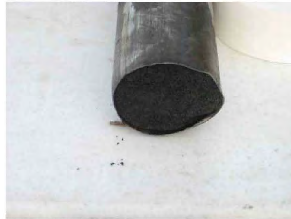
Photo 4. Soil filled core sampler prior to capping for shipment to the laboratory.
